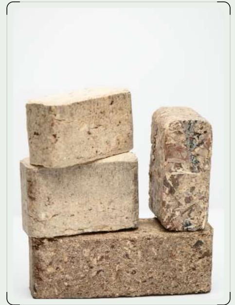
-- INERT CARBON BLOCKS CREATED BY GRAPHYTE TO STORE BIOMASS.
