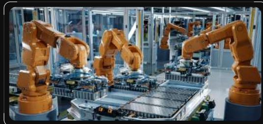
— ROBOTIC ARMS ASSEMBLING AN EV BATTERY PACK AT A COMMERCIAL SCALE PLANT
